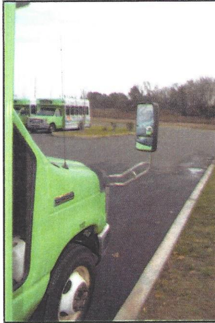
Photograph #6: Passenger side mirrors on the 2011 Ford Jitney bus (Writer's photograph)
